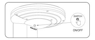
Press the key to turn on the projector and change the light color from 3000K to 4000K. When switching from one CCT to another, the device is switched off. The projector will turn on at dusk and will remain on until the battery runs out, the sun rises, or otherwise for up to 12 hours. The luminaire is equipped with a controller that automatically manages the light output as the night progresses and works as follows:
